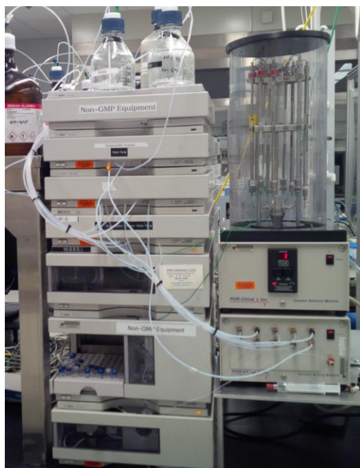
2 – AutoMDS on Agilent with older-style column selectors: 10 bottle/12 column HILIC on left and 10 bottle/24 column Chiral on right with one column selector for neutral and the other for acid additives.
