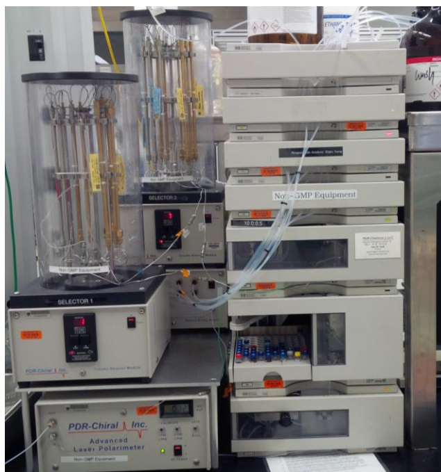
2 – AutoMDS on Agilent with older-style column selectors: 10 bottle/12 column HILIC on left and 10 bottle/24 column Chiral on right with one column selector for neutral and the other for acid additives.
