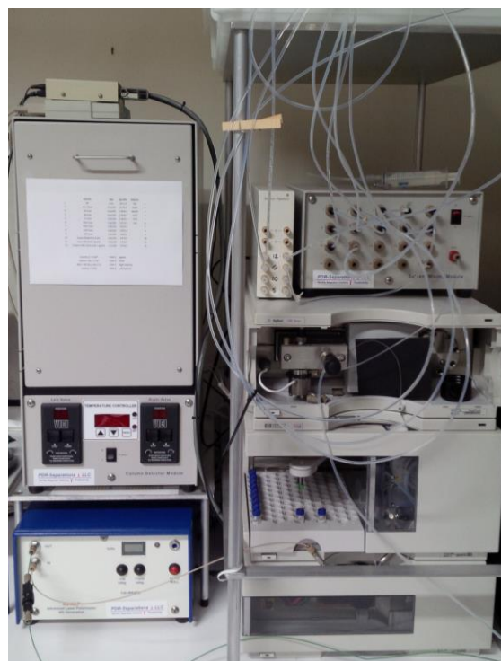
1 -- Method Development Plumbing and AutoMDS on Agilent with 20 bottles/24 columns with heating and cooling.
